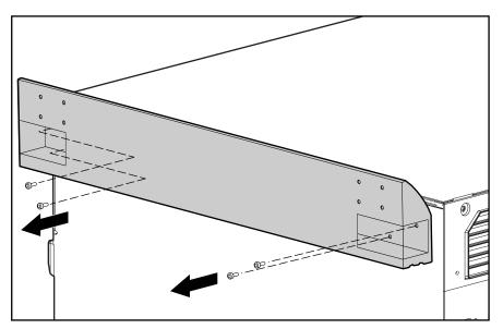
Figure 2-2. Removing the caster mounting support
